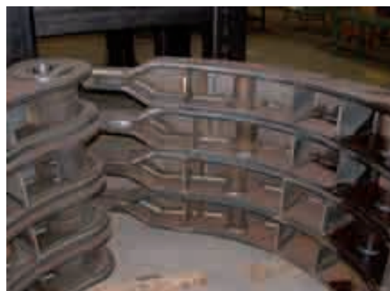
Figure 3. Detail of anti-twisting reinforcements in the shells of the claws
